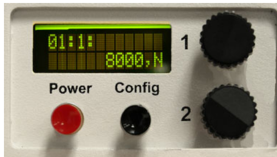
Close up of the LCD display, showing the board and channel on the top and the line length and communication settings on the bottom.
