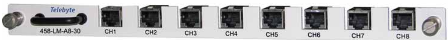
Figure 1: Front View of Model 458-LM-A8-30. Both the front and rear of the line module have 8 RJ-45 connectors.
